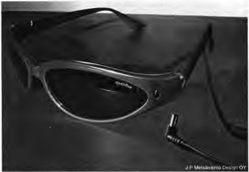
Figure 5. Augmented reality sunglasses are an optional CyPhone accessory. They can be used for more convenient viewing visual information.
